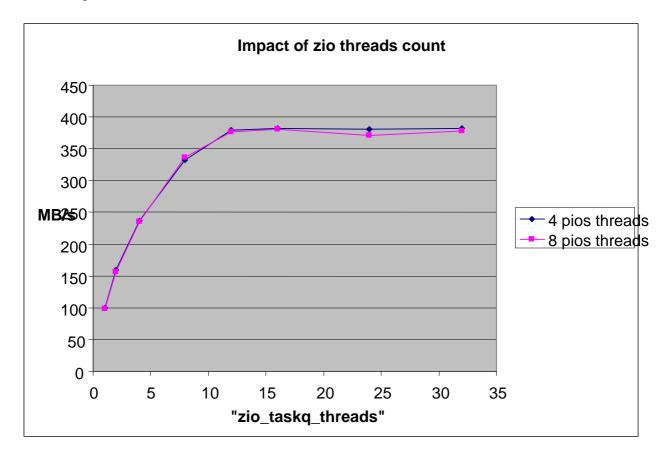
It first appears zio\_taskq\_threads count has a strong impact of ZFS' throughput. Also, the default value of 8 threads is not optimal. We get the best performance using at least 12 zio threads.
