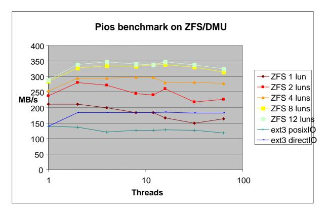
When doing a 'dd' command directly on such a device, we get about 350MB/s.
